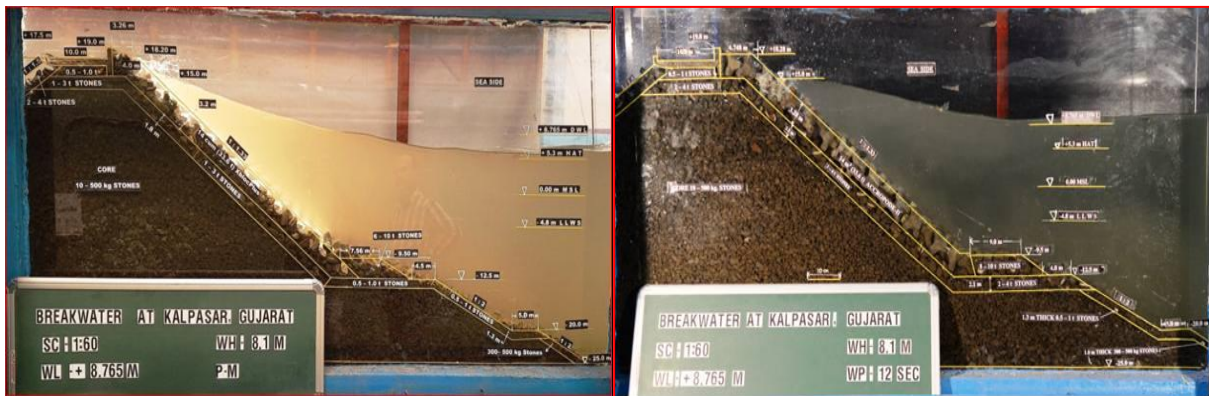
Fig.6.8 Wave action on the XblocPlus & Accropode-II armour units of sea dyke cross-section at -25.0 m bed level during (Hs) of 8.1 m at (DWL) of +8.765 m
