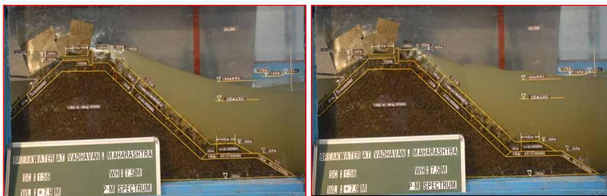
Fig 6. Wave action on trunk section armour layer (11 cum ACCROPODE™ II) at -19.0m bed level with wave height of 7.5 m at +7.9 m water level.
