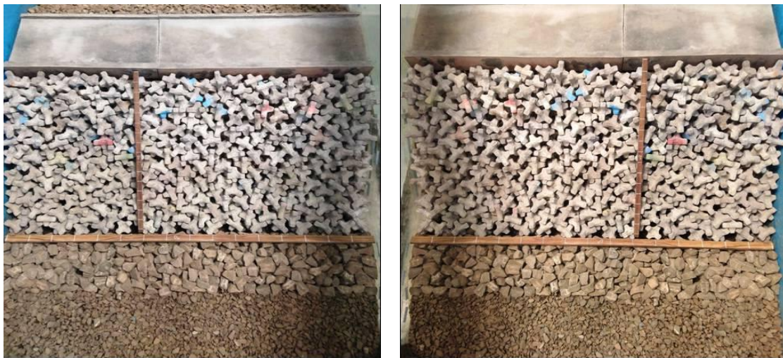
Fig.6.5 Placement of AccropodeTMII model units in the wave flume
