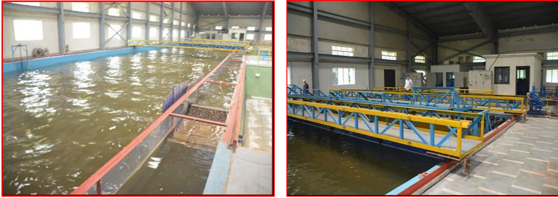
Fig.6.4 The wave flume facility with random wave generating system
