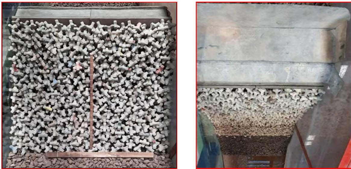
Fig 5. Placement of ACCROPODE™ II model units and arrangement of overtopping discharge tray.
